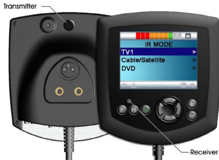
Figure 7 – Infra Red Transmitter, Receiver and User Screen
