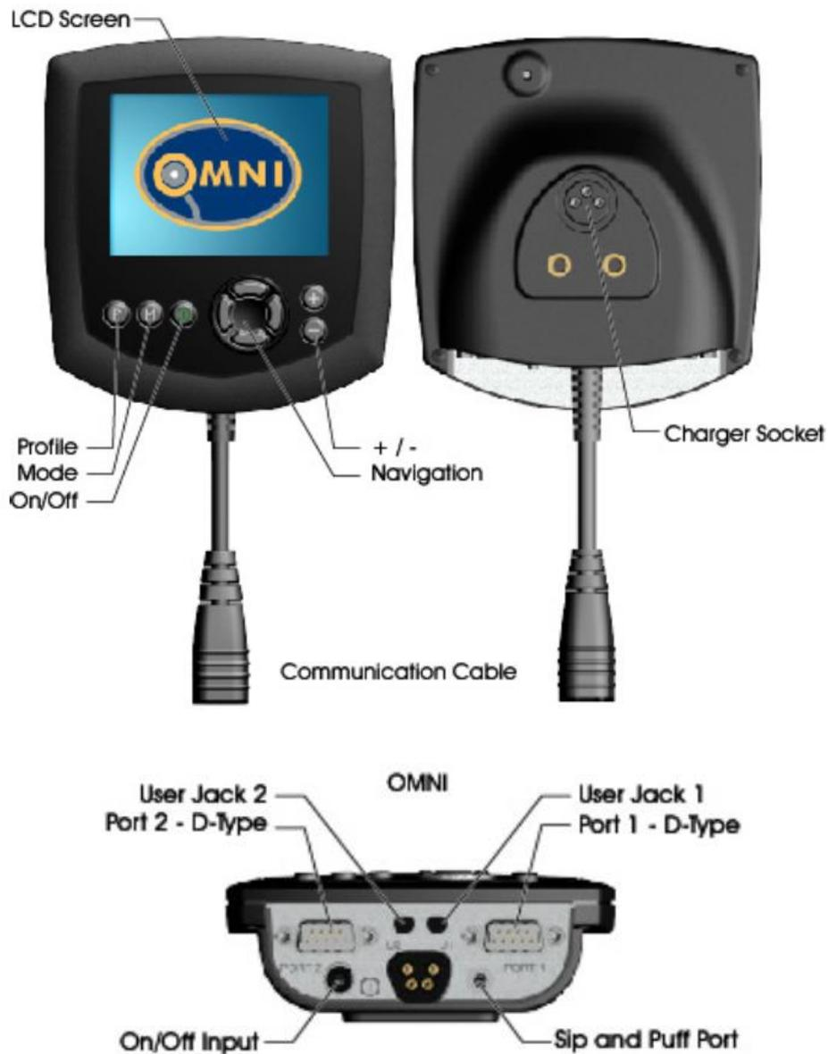
Figure 1 - Hardware: Controls and Connections
