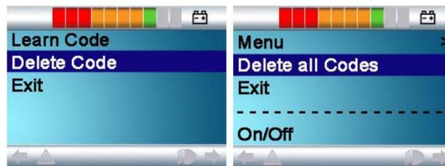
Figure 13 - Deleting individual IR Codes (left) and sets of IR Codes for an Appliance (right)
