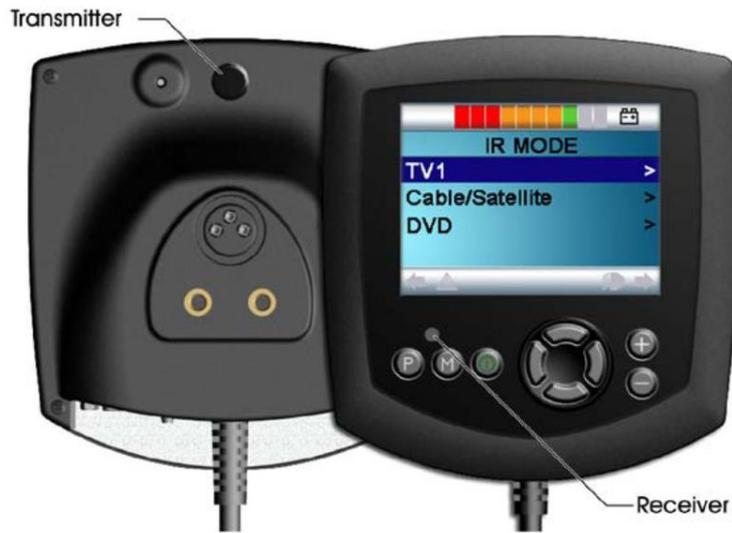
Figure 7 – Infra Red Transmitter, Receiver and User Screen
