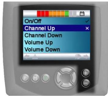
Figure 12 - Disabled and Enabled IR Codes
