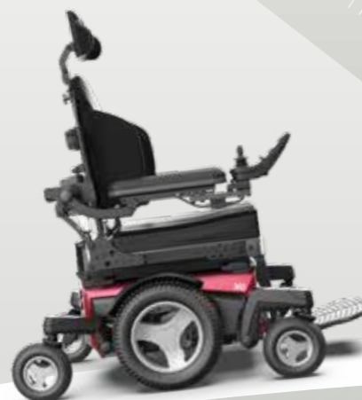
Urban 14" drive wheels for ultimate urban manoeuvrability (610mm / 24" wide)
