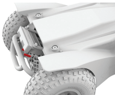
Figure 4.6a Extreme X8 brake levers engaged
