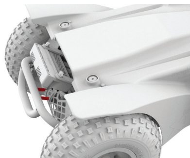
Figure 4.6b Extreme X8 brake levers released
