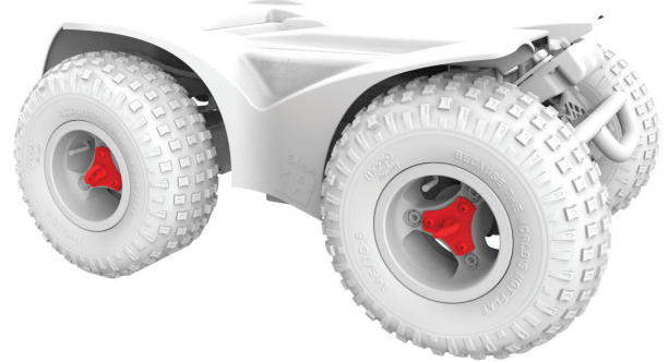
Figure 5.2d Extreme X8 lifting points (sold separately)
