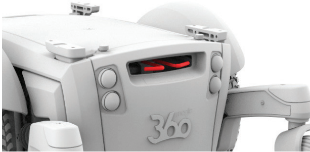
Figure 4.4a Magic 360 brake levers engaged
