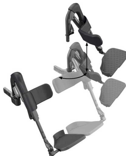
Figure 4.2c Swingaway Legrest showing removal action
