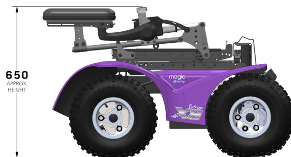
Figure 4.3d Extreme X8 Fold Forward height
