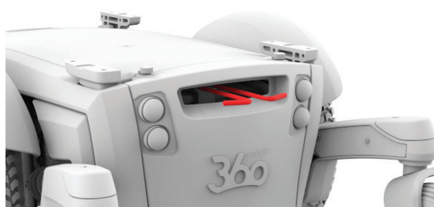
Figure 4.4b Magic 360 brake levers released
