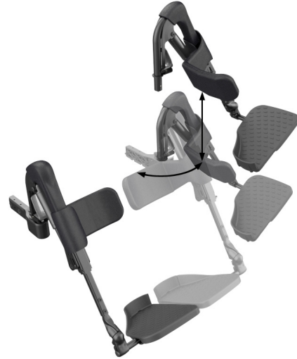
Figure 4.2c Swingaway Legrest showing removal action
