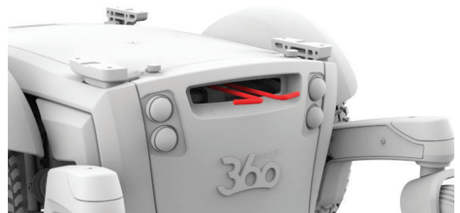
Figure 4.4b Magic 360 brake levers released
