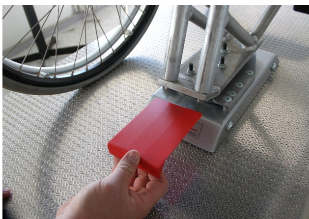
Figure 3: Emergency release tool
