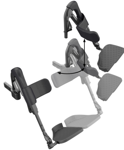
Figure 4.2c Swingaway Legrest showing removal action
