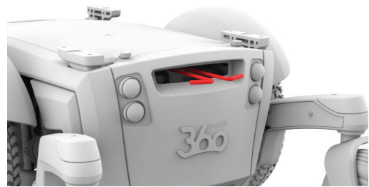
Figure 4.4b Magic 360 brake levers released
