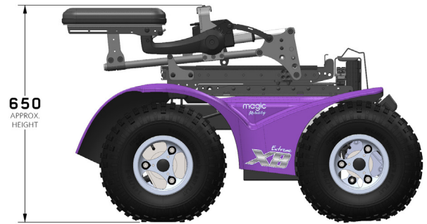
Figure 4.3d Extreme X8 Fold Forward height
