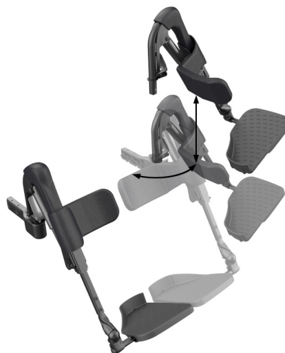
Figure 4.2c Swingaway Legrest showing removal action
