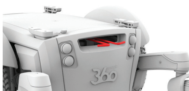
Figure 4.4b Magic 360 brake levers released
