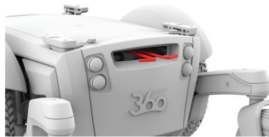
Figure 4.4b Magic 360 brake levers released
