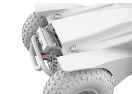
Figure 4.6b Extreme X8 brake levers released
