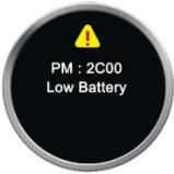
When the control system safety circuits have operated and the control system has been prevented from moving the wheelchair a diagnostics screen will be displayed.
