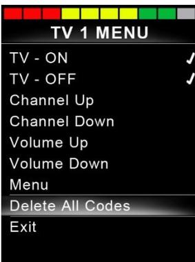
To delete all IR Codes stored in the CJSM2, select Delete All Codes within the IR Set-up Menu.
