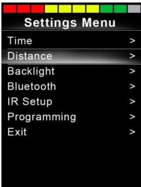
The Settings Menu allows access to user-related adjustments. The menu is accessed by depressing and holding the top left-hand Screen Button for 1 second. A typical Settings Menu display would be as above.
