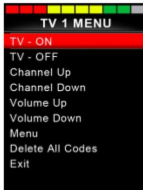
For each Appliance there is a list of associated IR Commands. Using the TV example, Commands such as: TV - ON, TV - OFF, Channel Up, Channel Down, Volume Up and Volume Down may be displayed. When the CJSM2 is transmitting the selected Command, it is highlighted with a red background.
